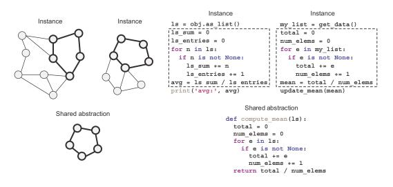
Figure 14.10 Program-centric analogy identifies and isolates isomorphic substructures across different instances
