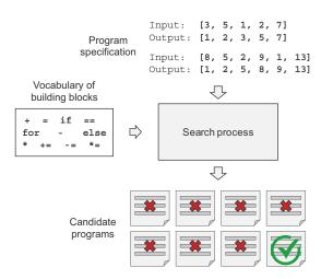
Figure 14.11 A schematic view of program synthesis: given a program specification and a set of building blocks, a search process assembles the building blocks into candidate programs, which are then tested against the specification. The search continues until a valid program is found.
